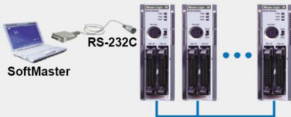
Remote connection using RS-485 Communication
