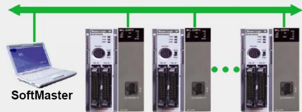
Remote connection using Ethernet
